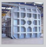
Electron-beam welding can be performed in large vacuum chambers whose volume is comparable to that of a singlefamily home.
